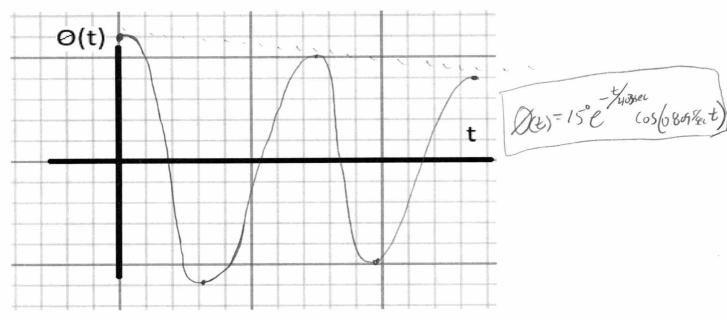
(3 pts) Now, Miley Cyrus (70 kg) jumps onto the wrecking ball to add a driving force to the pendulum and keep its motion from decaying. What driving angular frequency must she use for her force to optimize her efforts?
