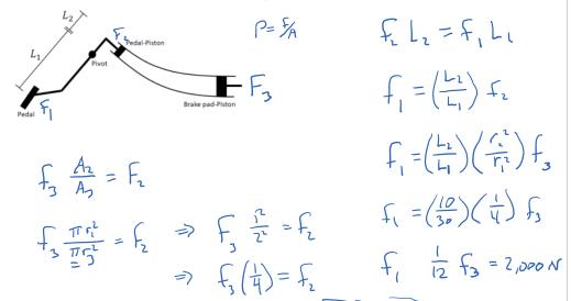
(b) If the density of brake fluid is 1,872  $\frac{kg}{m^3}$  and the pedal-piston is 150.0 meters above the brake pad-piston: what is the pressure in the brake fluid next to the brake pad-piston? Next to the pedal-piston?
