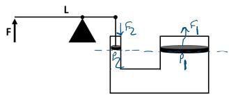
What hydraulic advantage does the piston system have if the larger piston has a radius of 32.0 cm and the smaller piston has a radius of 9.50 cm? (image may not be drawn to scale!)
