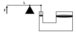
(a) What hydraulic advantage does the piston system have if the larger piston has a radius of 32.0 cm and the smaller piston has a radius of 9.50 cm? (image may not be drawn to scale!)
